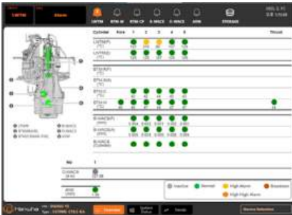
EDPD Monitoring System (Engine Driving Parts Diagnosis)
